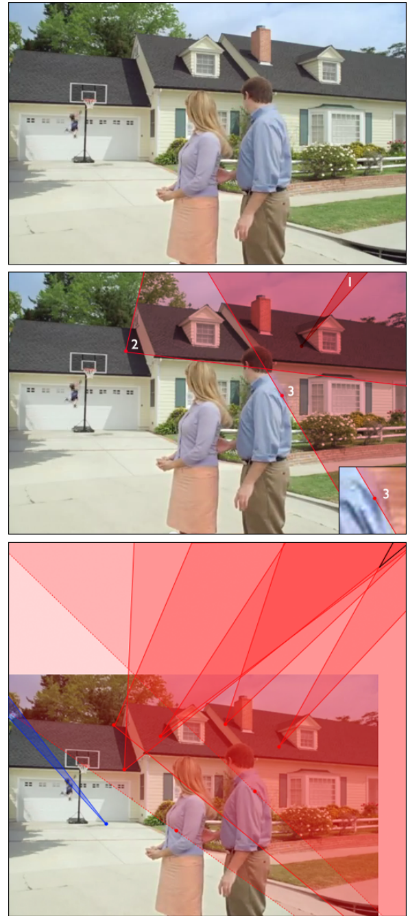
Fig. 2. Shown are: (top) a frame from the Geico commercial “Dunk – Easier Way to Save” depicting a somewhat incredible athletic performance; (middle) examples of cast (1-2) and attached (3) shadow constraints. The projected location of the light source must lie in the intersection of these constraints. Shown in the bottom is a multitude of constraints (solid lines correspond to cast shadows and dashed lines correspond to attached shadows). The shadows from the people and house are consistent with a light source located somewhere in the black-outlined region. The boy's shadow, however, is inconsistent with the rest of the scene.
